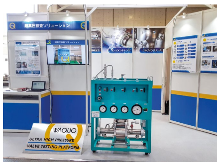
Ultra-high-pressure test bench for extreme condition valve integrity testing.
